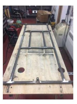
Weld all pieces together, as per drawing, ensuring all corners are square and chassis is level to base.
