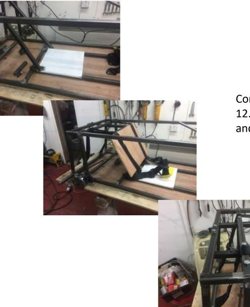
Construct Seat using 12.5mm ply, as per Drawing and cutting list
