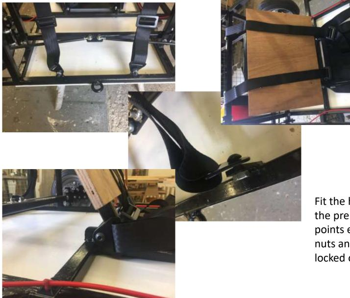
Fit the harness to the pre welded points ensuring all nuts and bolts are locked off and tight.
