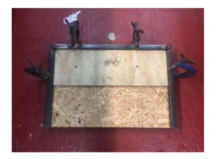
Take hoop bars from cutting list, weld together ensure square and equal, a quick template maybe of use as we have used here. Fit front and rear hoops to lower chassis, as per drawing. Ensure both are square and upright
