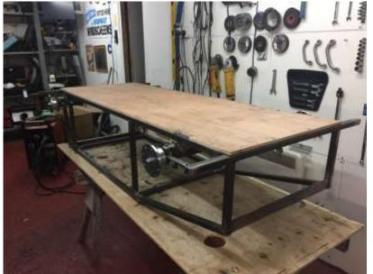
Turn Cart upside down and attach the 12.5mm ply as per drawing. Drill and tap all holes and use M6 panel fixings.
