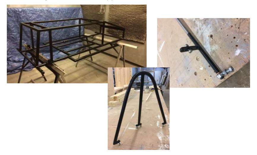
Preassemble all painted parts, loosely fit all nuts and bolts.
