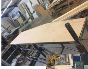
Cut and paint/spray body panel, metal, ply or any other suitable material may be used.
