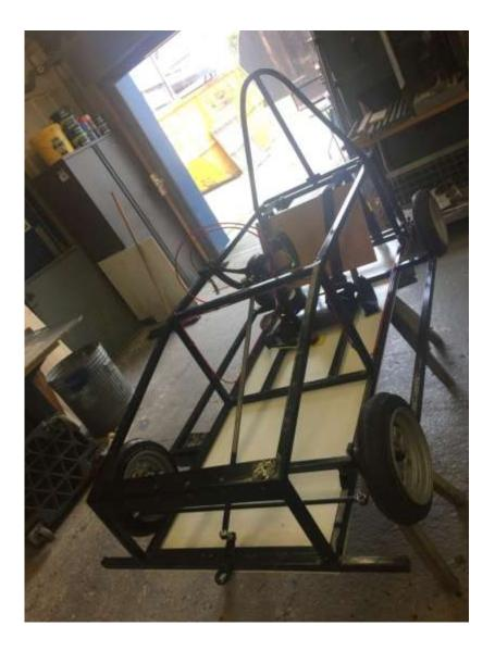
Assemble all parts together, along with running the brakes, ensuring they are clear the body panels, also allowing them to kink free. Left to left and right to right.
